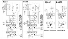
Electrical connections of heater BC
